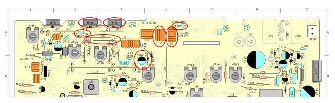
8) On the solder side of the radio PCB, remove C160 and C402. These parts are circled in red on the parts layout diagram below.
