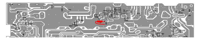
21) For S Series Radios with ERF2030 Finals Only – Do not perform this step on S Series Radios with 2SC1969 final transistors. Unsolder and remove the jumper wire located between the C171 and C208 PCB locations. Then unsolder the capacitor located at C209 and reinstall it at location C171. See diagram on next page.
